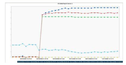
The temperature dropped from a starting point of 13.75 degrees in the office environment, to less than 8 degrees or so on site and the moisture content of the ground is rising steadily from 41% to 43.5% expressed volumetrically.
