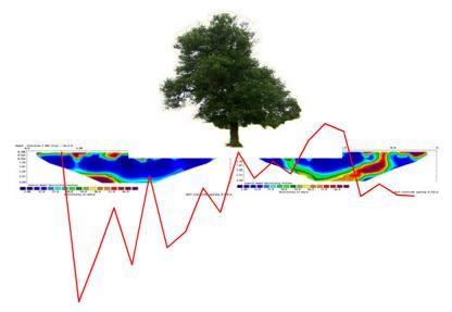
Station 21 has always been a 'high spot', moving less than its neighbours and we see in the ERT values the dark blue associated with rehydration in this location, and immediately to the right of this, at Station 22 and 23, the oranges and reds associated with dry soil where the levels confirm greater subsidence and slower recovery. Maximum movement recorded was 34.8mm at Station 9.
