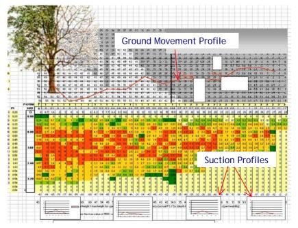
The model estimates ground movement of between 70mm close to the tree, reducing to less than 20mm or so at its 'root influence zone' periphery and below we have extracted the ground movement profile from the image above to clarify this.
