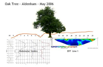
We now have a moving image of moisture change by month, from April, throughout the summer and the associated ground movement. Below is the September ERT image from array 2 of the Oak and we see the resistivity changing from a saturated mid to dark blue (May) to a deeper purple, as we would expect as the ground dries.
